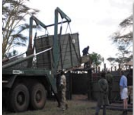
The Multilift system in Namibia (top) and the KWS “Hannibal” system in Kenya (bottom) are used to load/unload crates.
