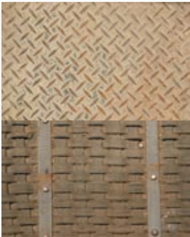
Steel “fish plate” (top) and woven rubber matting (bottom) give good footing in a transport crate.
